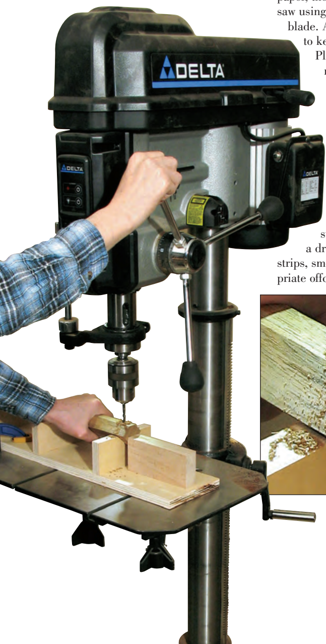
A shop-made cradle jig with a registration stop will help to ensure that the screws and countersinks are perfectly positioned and drilled.
