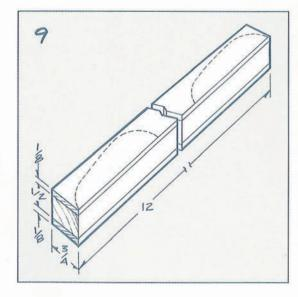
Scribe a line connecting the semi-circular holes in each side as shown by the dotted line. Also, using a compass, scribe a 1 in. radius on each upper corner. Make the cuts with a band saw, then sand the edges smooth.
